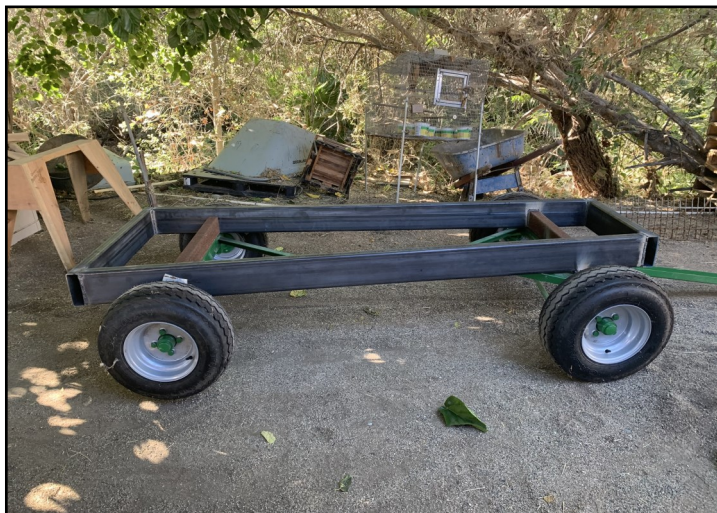
2. Trailer chassis welding complete
