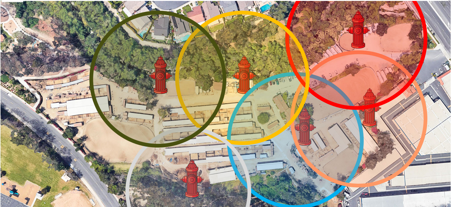
Aerial Photo #2- Coverage area from each hydrant
