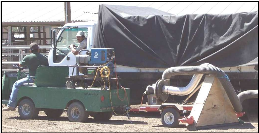
Shown here is the first run of the prototype arena vacuum. The black fabric on the truck was later replaced with a giant sealed dust bag to eliminate dust leakage.
